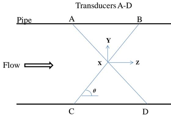
Figure 1: Two pairs of transducers (A–D) are placed in the flowmeter body with the transducer centerlines inclined at an angle to the flow direction
