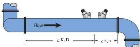
Figure 2: Transducers positioning
