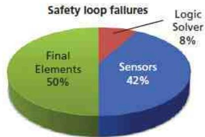
Adding diagnostic test features on the components, in order to take preventive measures and ensure availability of safety system, would have positive impact on the system SIL. After installing the HIPPS, various test at specified intervals shall be carried-out as recommended by SIS integrator in order to maintain the required SIL.
