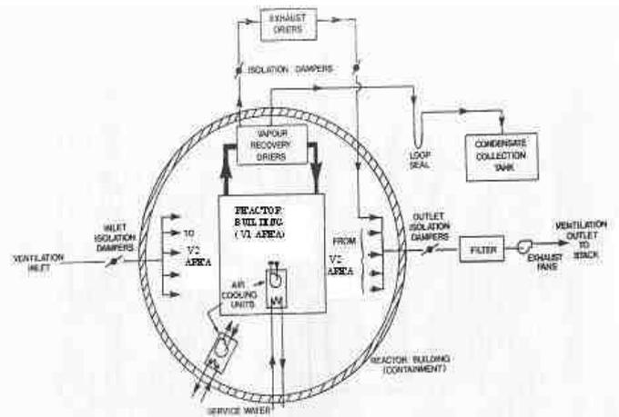
Fig.1 Typical Containment Ventilation and Cooling System
