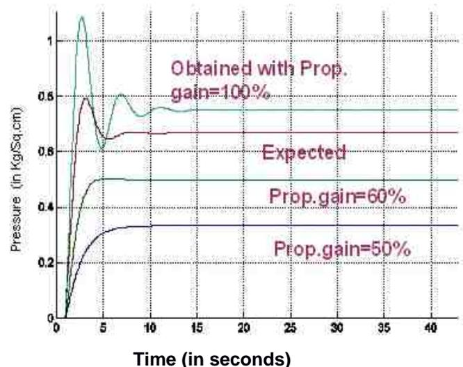
Fig.9 Performance characteristics using Proportional Control
