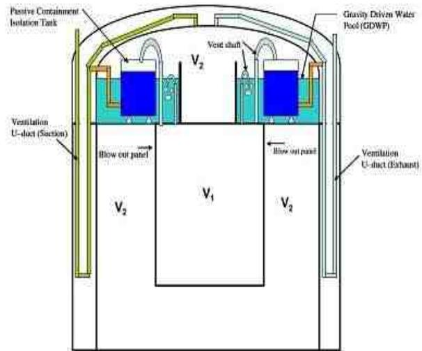
Fig.2 Schematic of Passive Containment Isolation System
