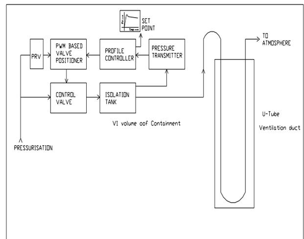
Fig.5 Set up for studies on Passive Containment Isolation
