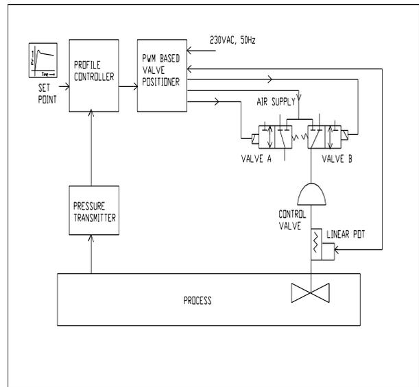
Fig.7 Electro-pneumatic Valve Positioner with on/off solenoid valves
