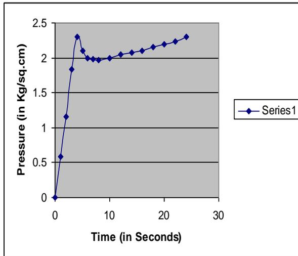
**Fig. 6 Expected pressure transient for studies on containment isolation**
