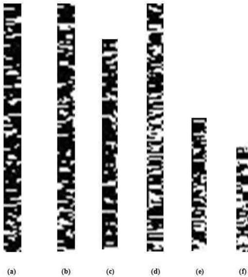
**Figure 11- Image processed output data for different void fractions (a)  $\alpha=11\%$  (b)  $\alpha=20\%$  (c)  $\alpha=33\%$  (d)  $\alpha=42.85\%$  (e)  $\alpha=50\%$  (f)  $\alpha=55.5\%$ .**
