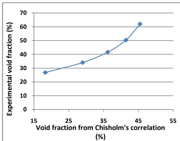
Figure 9- WMS experimental Vs Chisholm's correlation void fraction data
