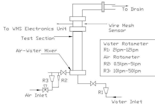
Figure 2- Schematic drawing of WMS Experimental Test Facility
