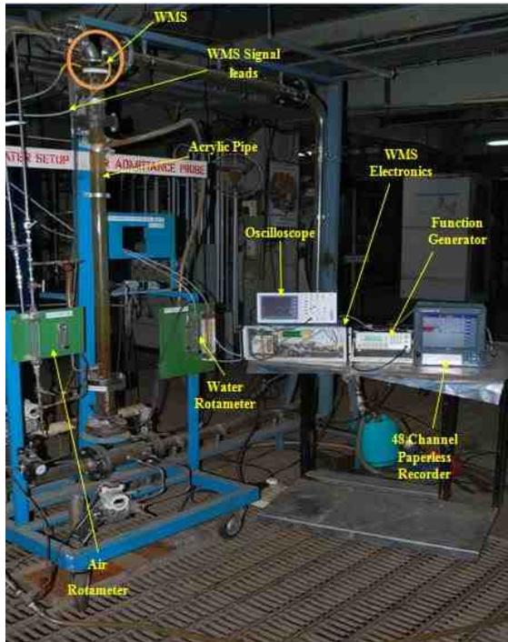
**Figure 3- WMS experimental setup with sensor electronics**
