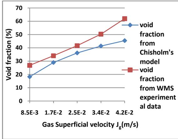
Figure 8- Void fraction from the Chisholm's model and WMS experimental data for different gas superficial velocities
