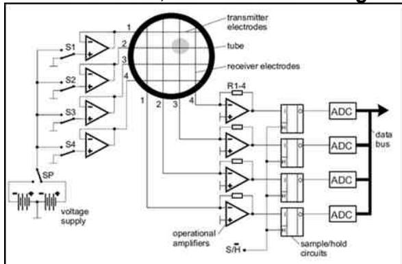
Figure 1- Simplified scheme of a two 4X4 WMS with signal acquisition system
