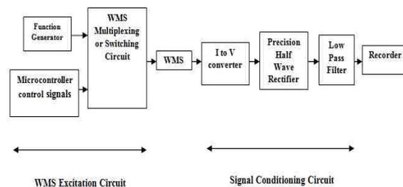
**Figure 5- Block diagram of WMS electronics**
