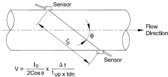
$$V = \frac{l_0}{2 \cos \theta} \times \frac{\Delta t}{t_{up} \times t_{dn}}$$
