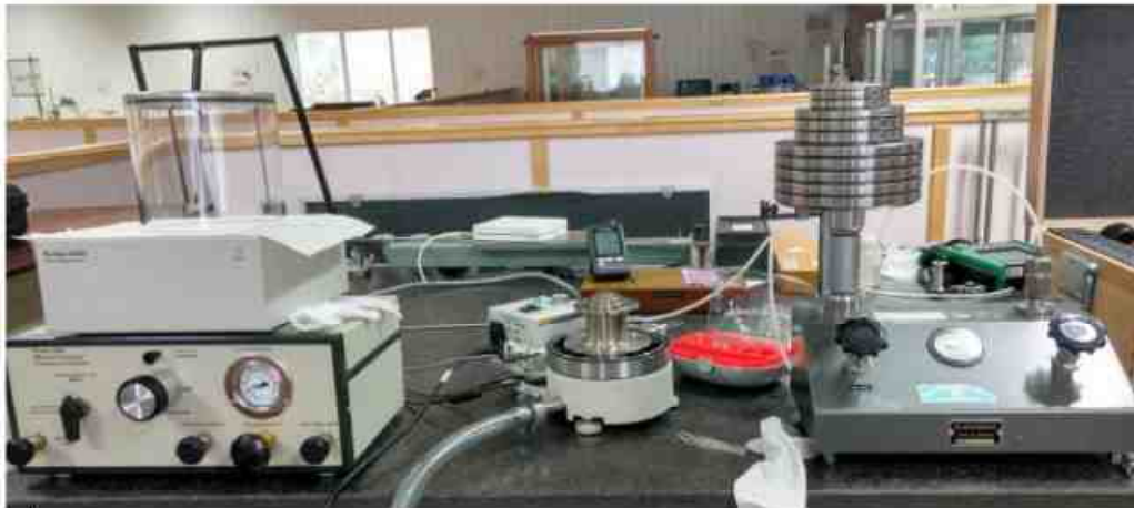
Fig.1 Ruska 2465 Piston Gauge used for the determination of Effective Area of (0.25 to 7) bar g Air Dead Weight Tester
