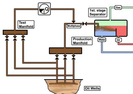
Figure 6. Multiphase meter replacing test separator and its meter [4]
