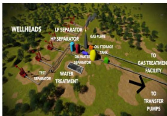
Figure 1. Typical Conventional Facilities for Crude Oil Production
