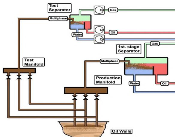
Figure 5. Conventional well testing using test separator [4].
