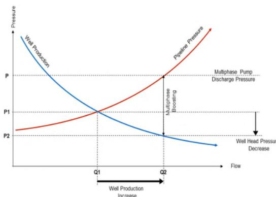
Figure 3. Well production increase due to multiphase boosting
