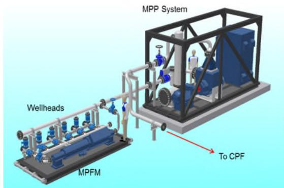
Figure 7. Smart system combining MPP and MPFM.
