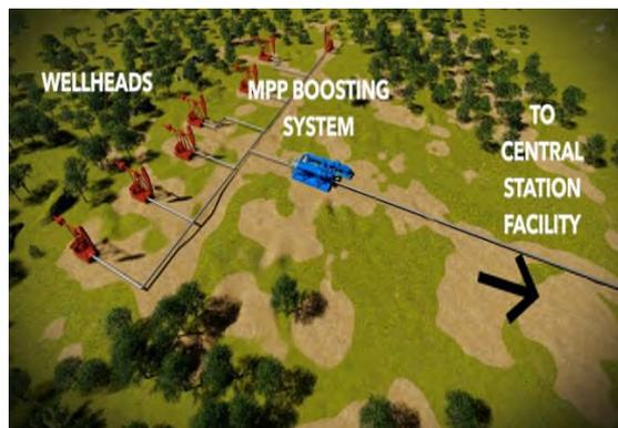
Figure 2. MPP System for crude Oil Production
