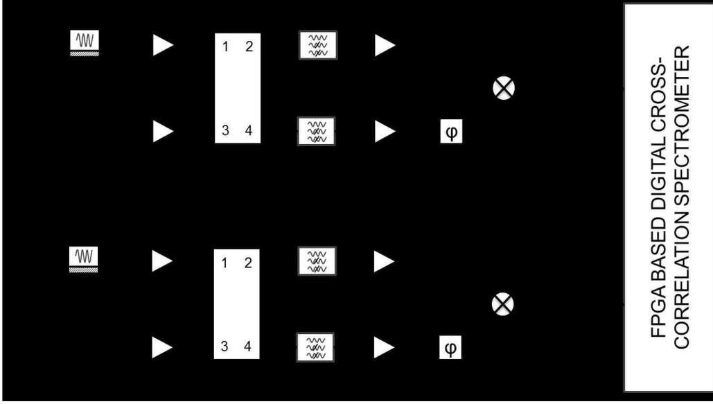
**Figure 2:** Correlation Radiometer design for measuring temperature difference in the water in the high-pressure and low-pressure sections (i.e. upstream and downstream) of the turbine.
