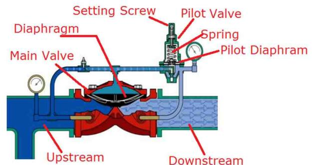
Fig-2. Working Principle of Self Actuated Pressure Regulator.
