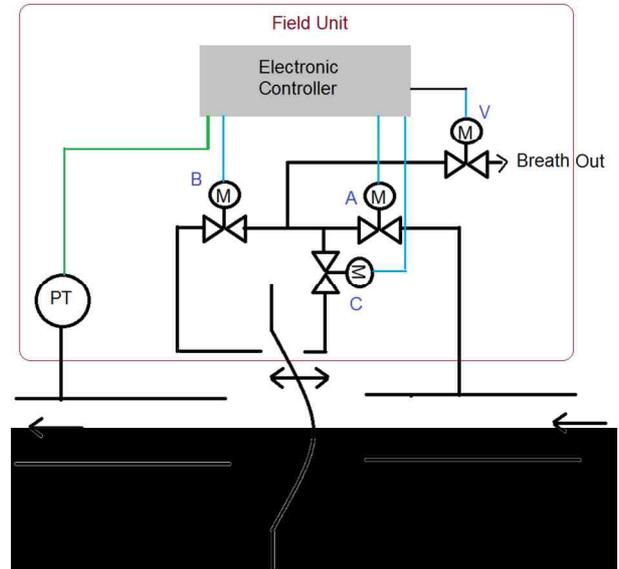
Fig-4 Schematic Diagram of Servo Pilot
