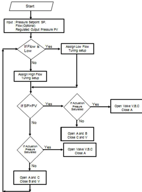
Fig-5 Flowchart of Controller Algorithm
