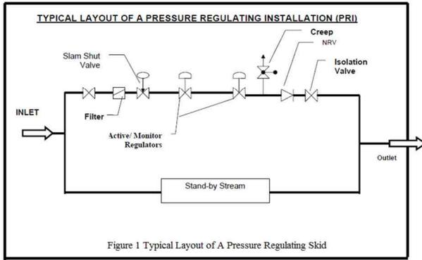
Figure 1 Typical Layout of A Pressure Regulating Skid
