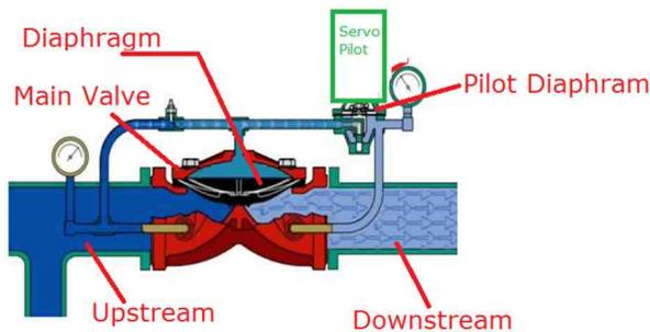
Fig-3. Servo Pilots for Pressure Regulators
