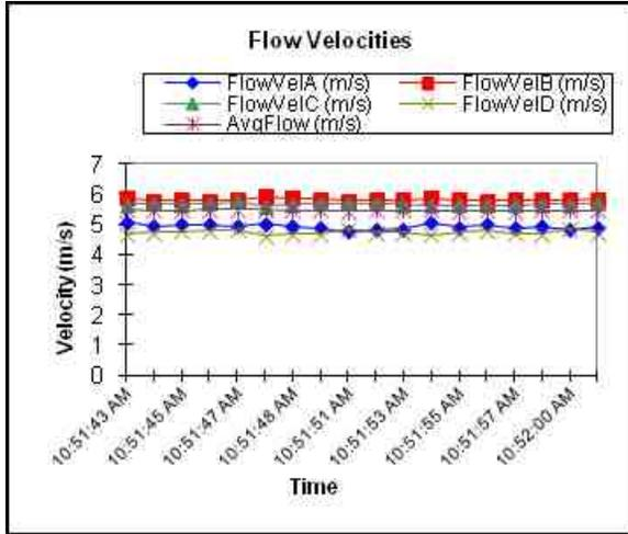
Fig.7 Comparison of chord flow velocities
