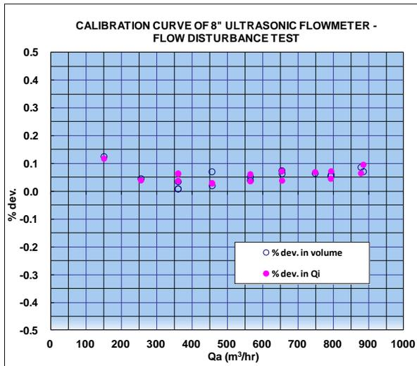
Fig.11. Calibration curve with flow disturbance test.
