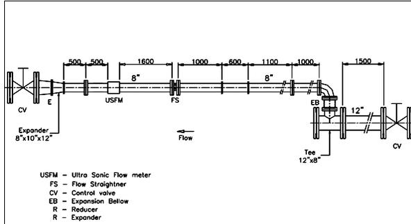
Fig.10. Schematic of test set up for disturbance test
