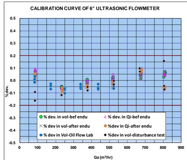
Fig.13. Calibration curve of 6" ultrasonic flowmeter
