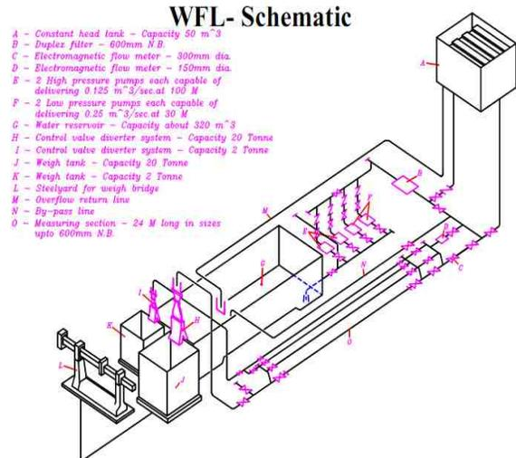
Fig.1 – Schematic of Water Flow Laboratory
