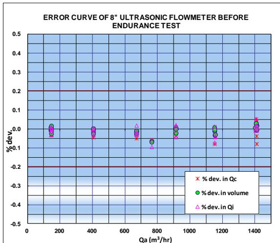
Fig.8. Calibration curve before endurance test
