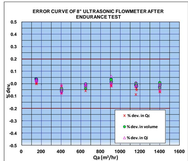
Fig.9. Calibration curve after endurance test
