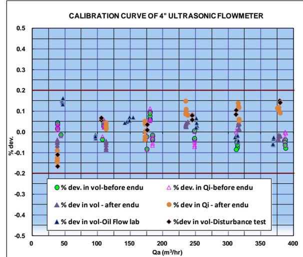
Fig.12. Calibration curve of 4" ultrasonic flowmeter
