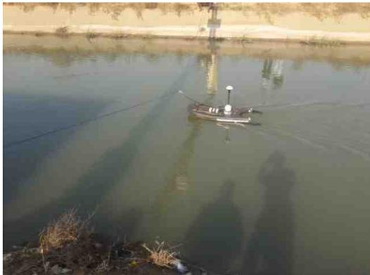
Figure 3 Contact free radar sensor being calibrated with ADCP
