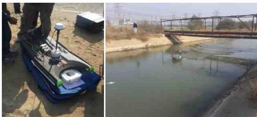
Figure 8 ADCP arrangement at site
