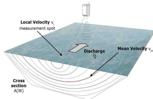
Figure 2 Principle of RQ30A sensor
