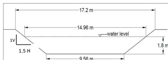
Figure 7 Cross section of DSB
