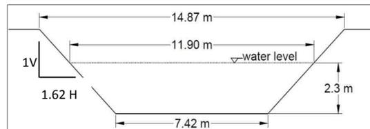
Figure 6 Cross section of CLC
