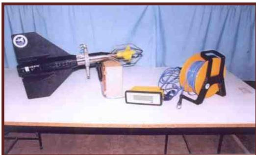
Figure 4 A view of propeller type current meter
