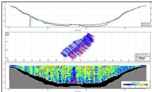
Figure 9 Pixel data of ADCP
