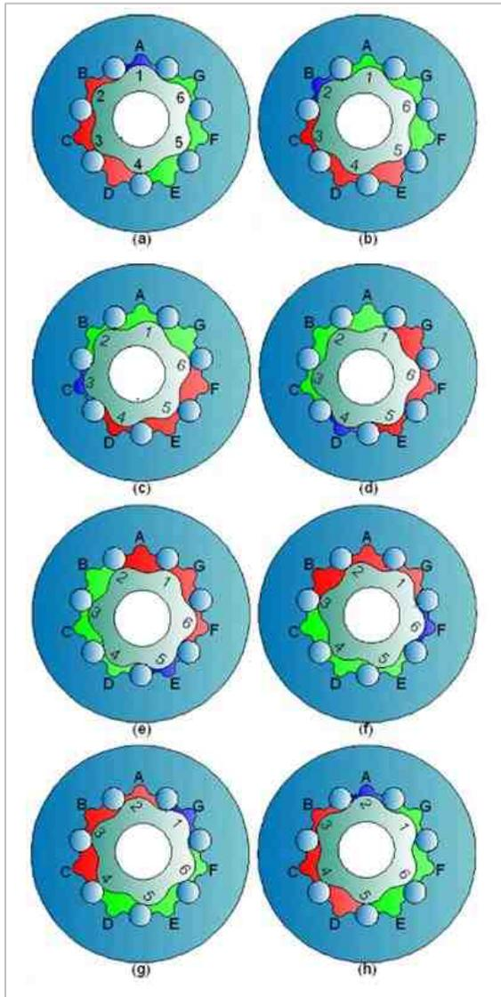
Figure 1-Geroler motor working principle
