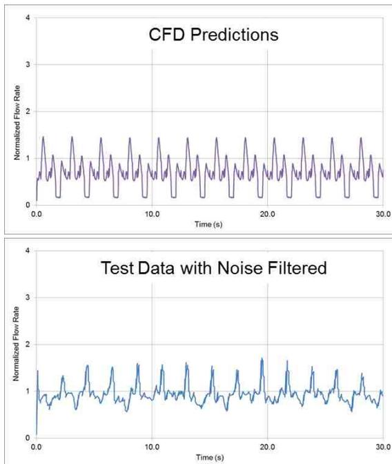
Figure 11-Simulation results validation with test data
