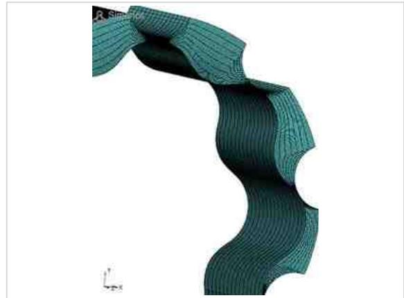
Figure 5-Structured mesh in deforming zone
