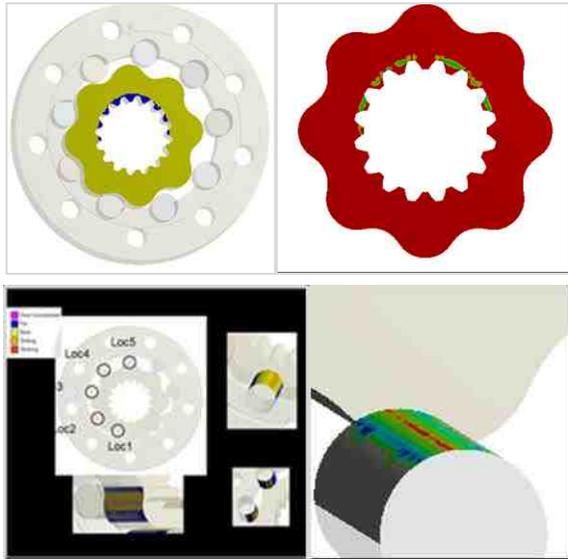
Figure 10-Axial and radial deformations from FEA
