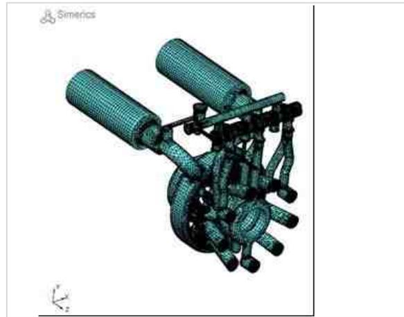
Figure 4-Non-deforming zone mesh in Geroler motor model
