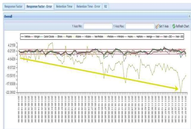
Fig. 19 C7+ response factor descends over time due to low pressure in calibration bottle
