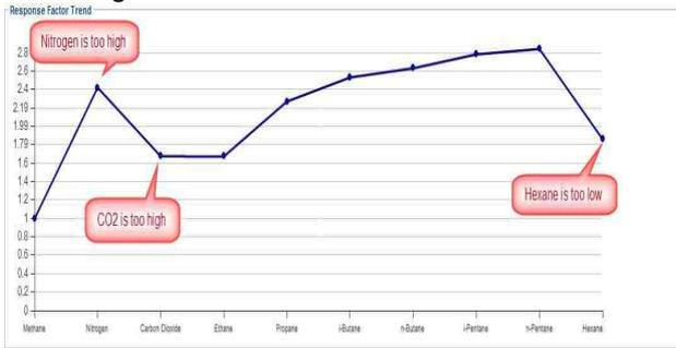
Fig. 15 - RF trend after component data table was adjusted
