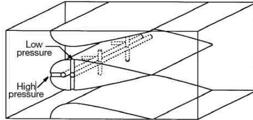
**Fig. 1 Aerofoil Pressure ports**
