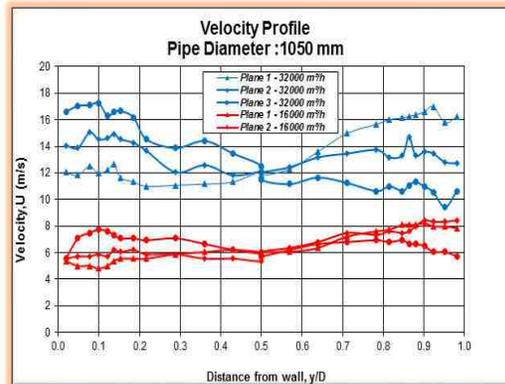
Velocity profiles in a rectangular cross section under different conditions.
