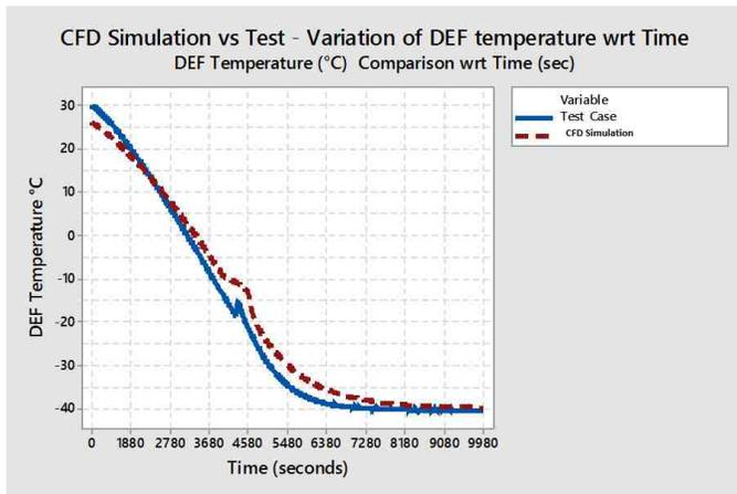
**Figure 8 CFD Simulation results comparison with Test data**
