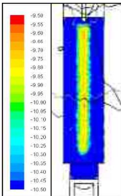
**Figure 9 Static Temperature Contour Plot showing DEF freeze behavior in cylindrical tube**
