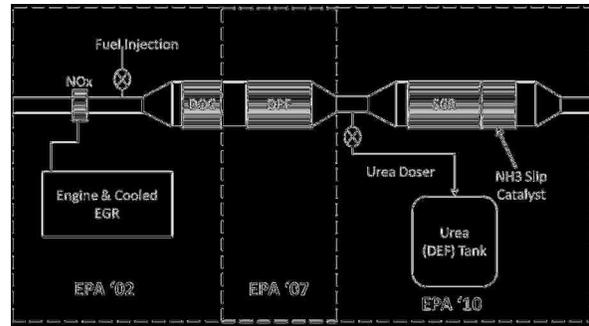
**Fig 1- Evolution of after-treatment system as per EPA norms**
