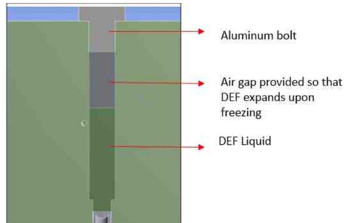
Fig 7 Simplified model considered for validation with test
