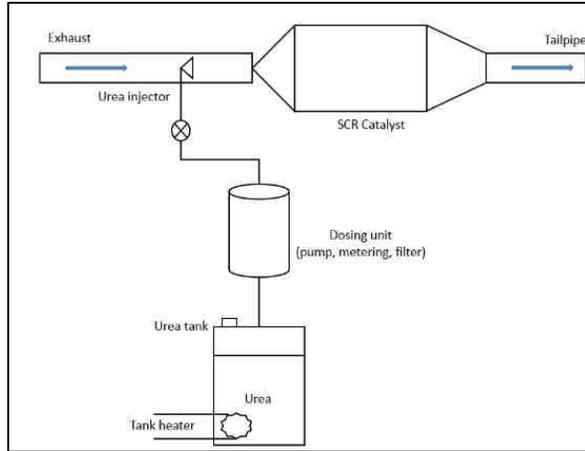
**Fig 3- Schematic diagram of an SCR system**
