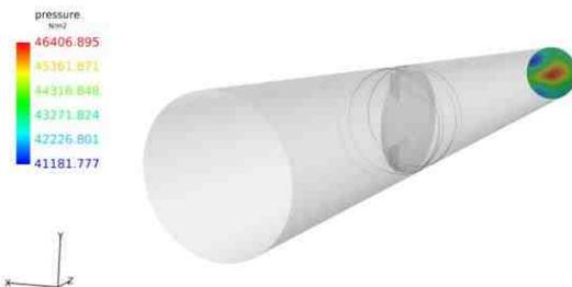
Fig 5-Pressure at Outlet
