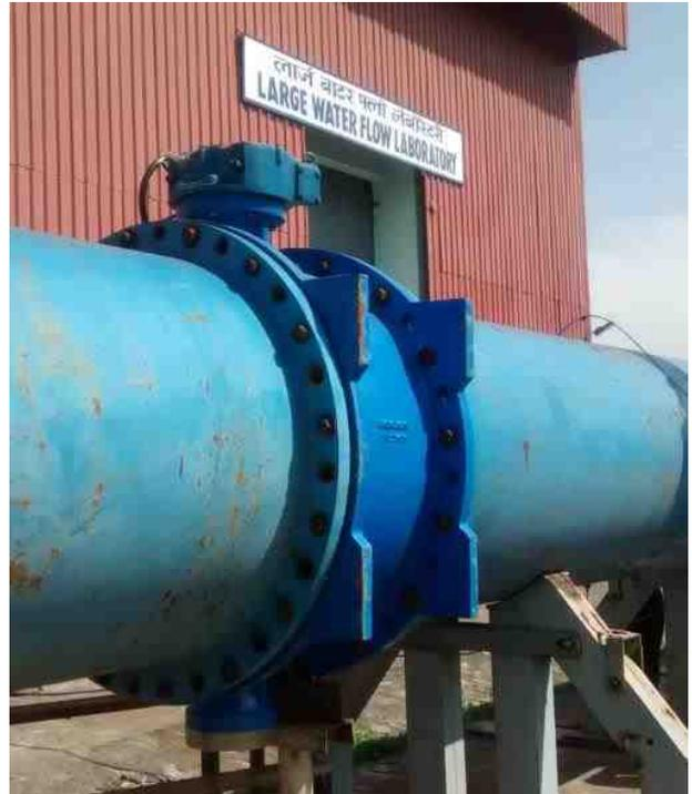
Fig 2- Butterfly valve at test line
