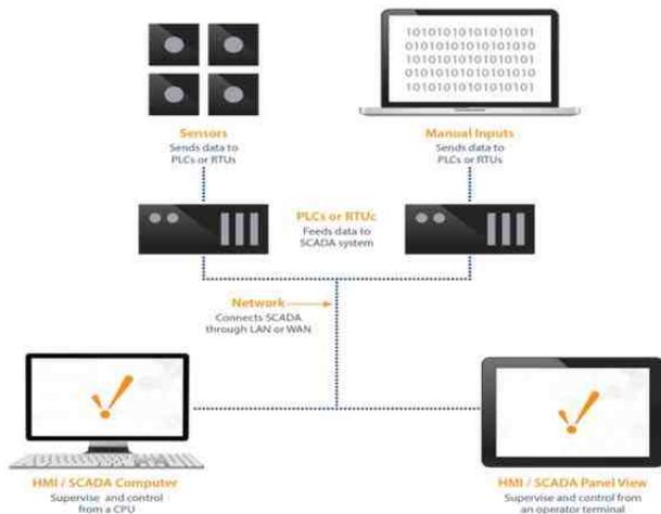
Figure 1 - Architecture of SCADA system.
