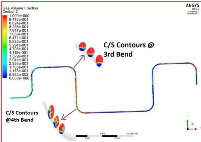
**Figure 4. Gas Volume fraction contours at mid plane**
