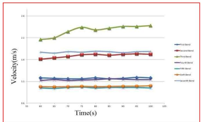
**Figure 19. Velocity across each bend for the mixed flow**
