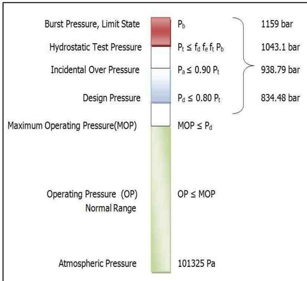
**Figure 2. . Design and Working Pressure**
