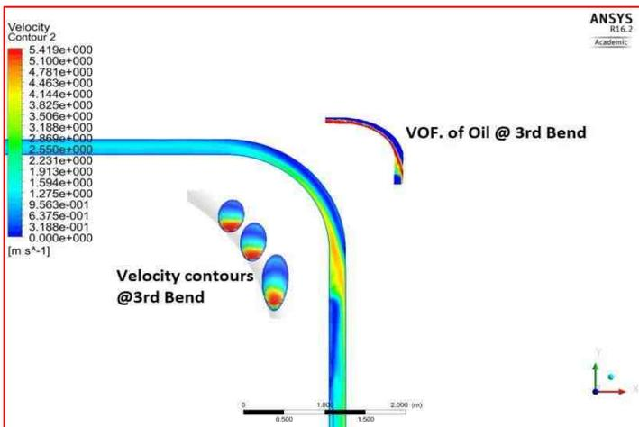
**Figure 5. The oil velocity contours at mid-plane**
