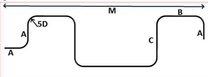
**Figure 1. M-shaped Jumper Geometry**
