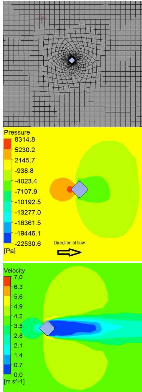
Figure 4 Typical Meshing, Pressure contour and velocity contour profile across the annubar
