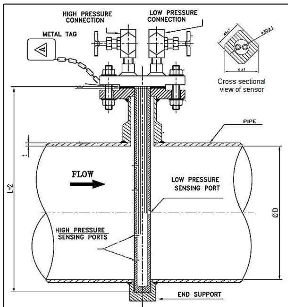
Figure 3 Typical annubar arrangement inside a pipe
