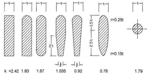
Figure 1 - Bar profiles as per IS 11388:2012.
