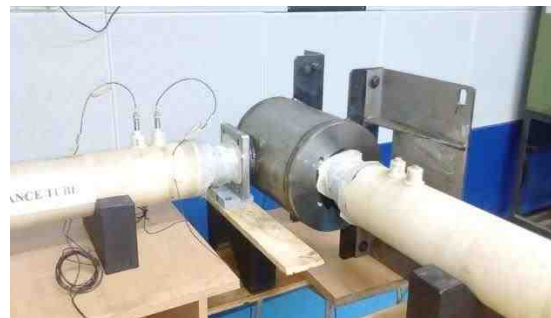
Figure 10 TL measurements in acoustic Impedance test facility
