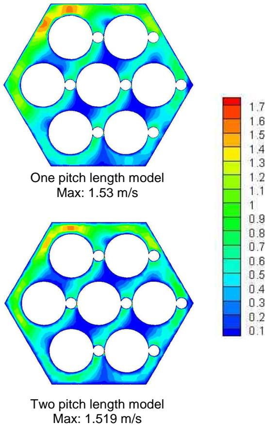
**Figure 13 - Comparison of cross-flow velocity (m/s) for 7 pin bundle with one pitch length and two pitch lengths**
