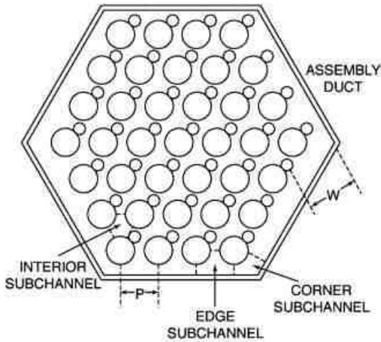
**Figure 3 - Various sub-channel flow areas in a subassembly**
