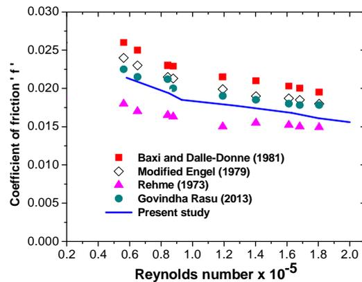
Figure 9 - Comparison of numerically predicted frictional factor with correlations proposed by various studies
