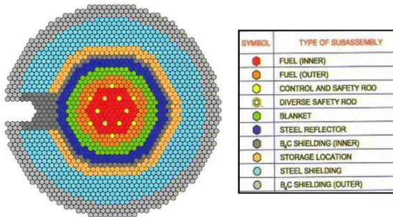
**Figure 1 - Core structure of PFBR**
