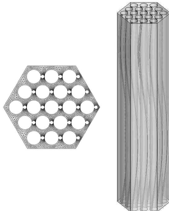
**Figure 14 – Mesh and 3-D view of 19 pin bundle model**
