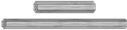
**Figure 12 - 3-D view of 7 pin fuel bundle model with one pitch length and two pitch lengths**
