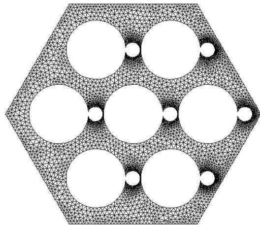
Figure 7 - Mesh for CFD model
