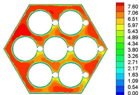
**Figure 11 - Vertical velocity (m/s) at the outlet ( $Re = 0.85 \times 10^5$ )**
