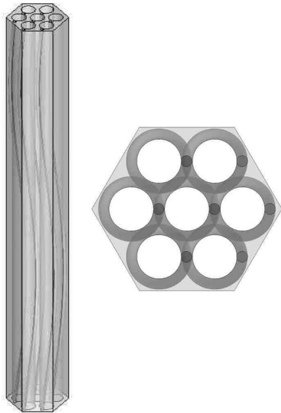
**Figure 5 - Computational model of 7 pin bundle**
