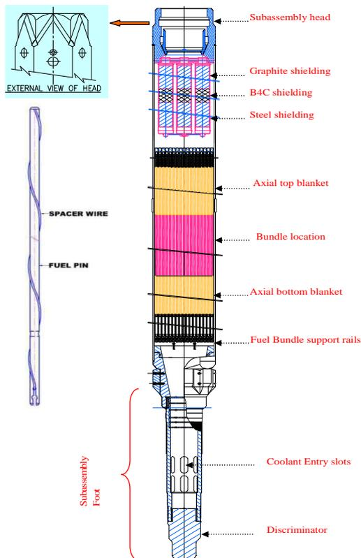
**Figure 2 - Structure of a typical fuel subassembly in FBRs**
