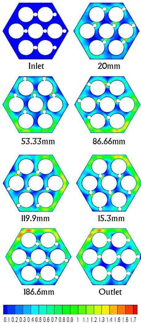
**Figure 10 - Cross flow velocity (m/s) development in the 7 pin fuel bundle from inlet to outlet**
