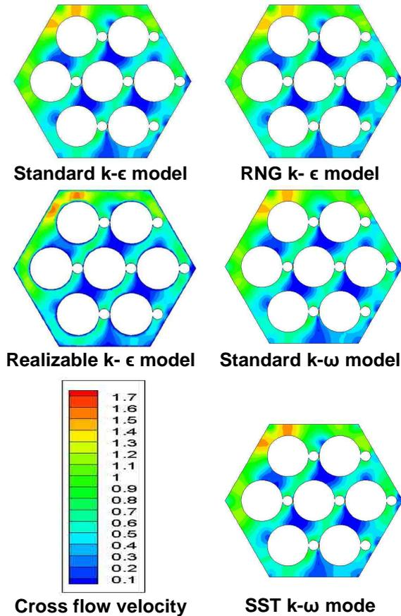
Figure 8 - Comparison of turbulence models
