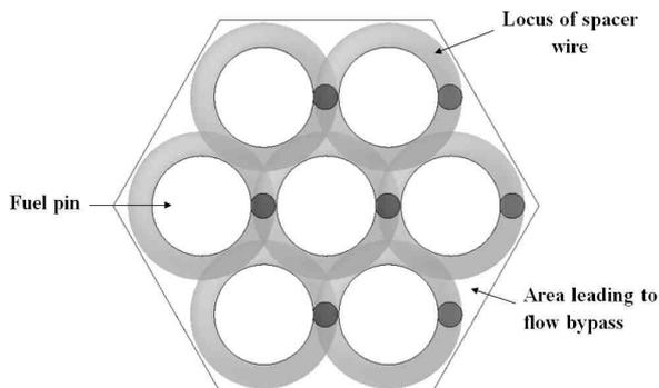
**Figure 4 - Flow bypass area in a fuel subassembly**
