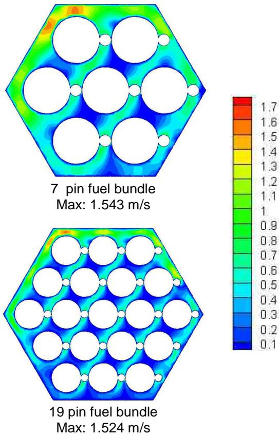
**Figure 15 - Comparison of cross-flow velocity (m/s) at the outlet for 7 pin and 19 pin bundles**
