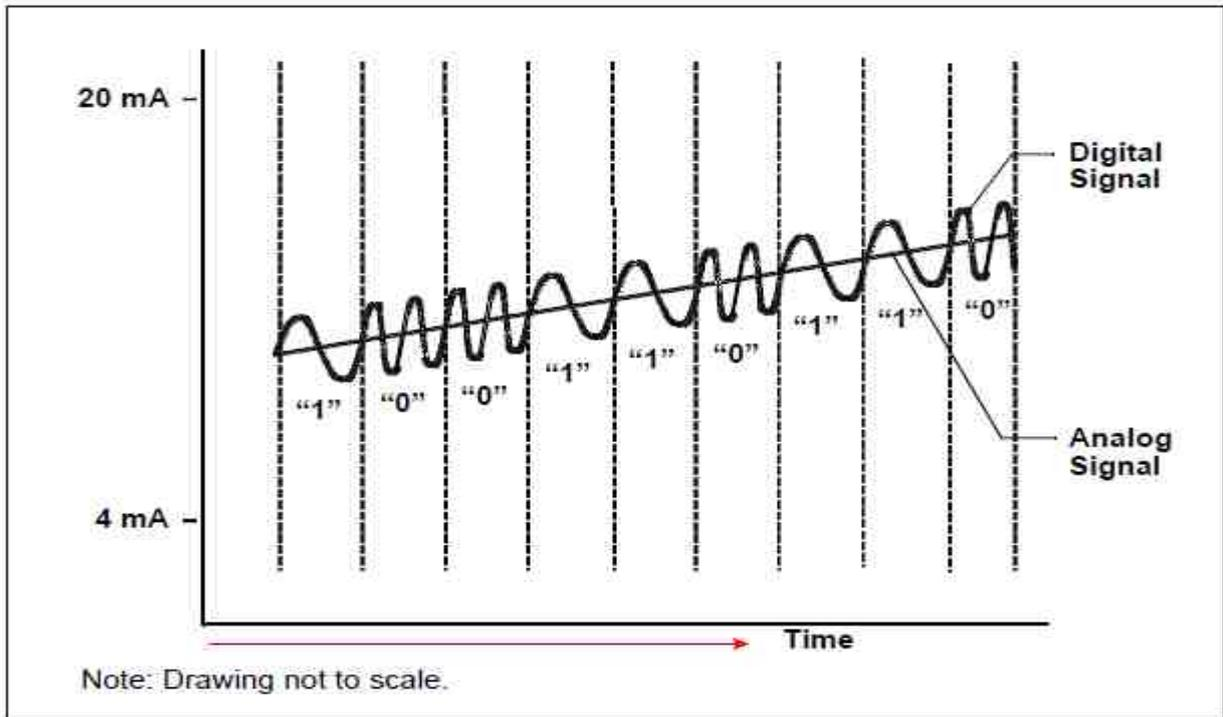
**Figure:2 Simultaneous Analog and Digital Communication**
