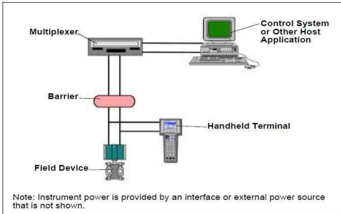
**Figure:3 Point to Point Mode of Operation**
