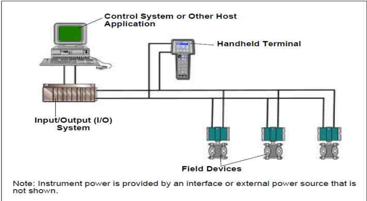
**Figure:4 Multidrop Mode of Operation**
