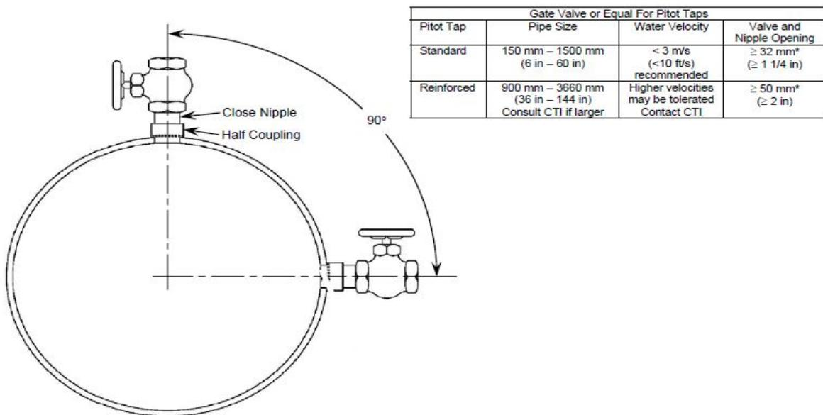
Figure 4: Pitot tap location [plan view]
