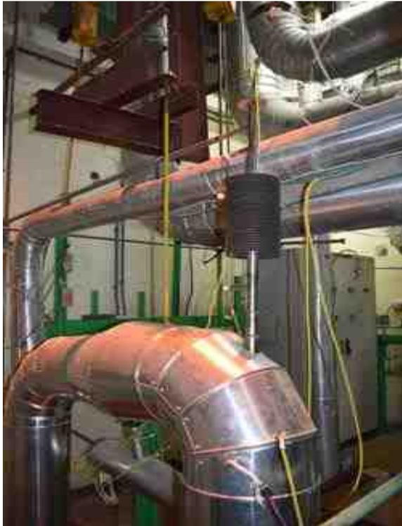
Figure 5 - Photograph of PPFMS Test section in SGTF
