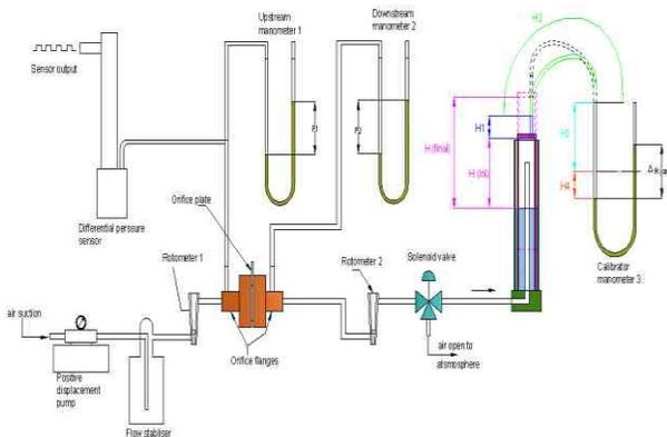
**Figure 3 - Experimental setup for demonstration of orifice meter with positive displacement pump.**
