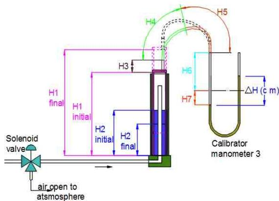
**Figure 4 - Experimental setup of calibration.**
