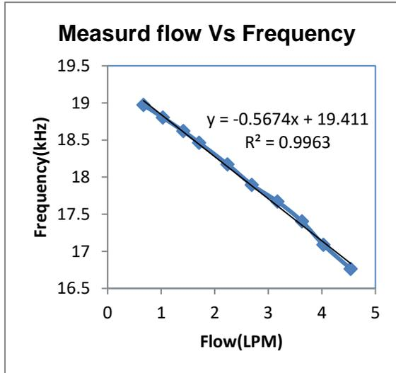
**Figure 6 - Sensor output freq. against flow using calibrator (Argon cylinder).**
