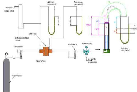
**Figure 2- Experimental setup for demonstration of orifice meter with Argon cylinder.**
