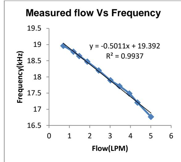
**Figure 7 - Sensor output freq. against flow using calibrator (positive displacement pump)**
