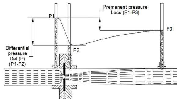
Figure 1- Pressure drop across an orifice
