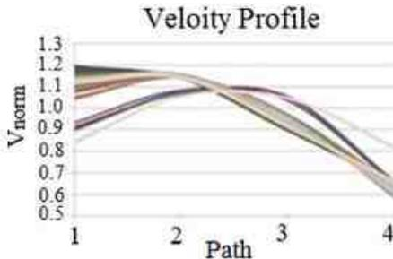
Fig 6. USM Diagnostics Field Result
