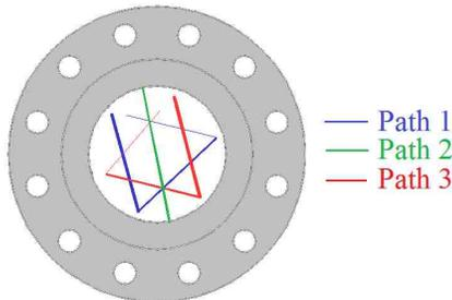
Fig 21. 8" Bounce Path Configuration
