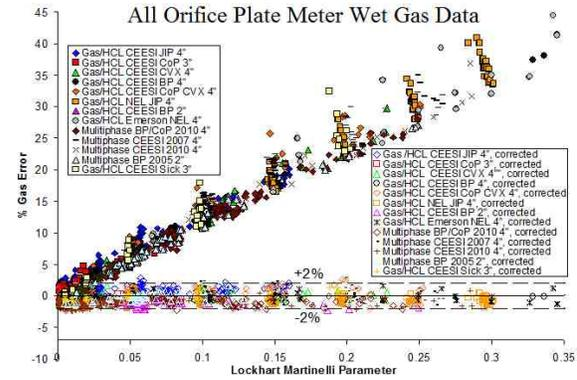
Fig 12. Massed 2" to 4" Orifice Meter Wet Gas Data With & Without the ISO Correlaton.
