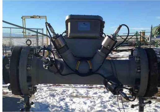
Fig 17. 8" 3 Bounce Path USM Wet Gas Testing
