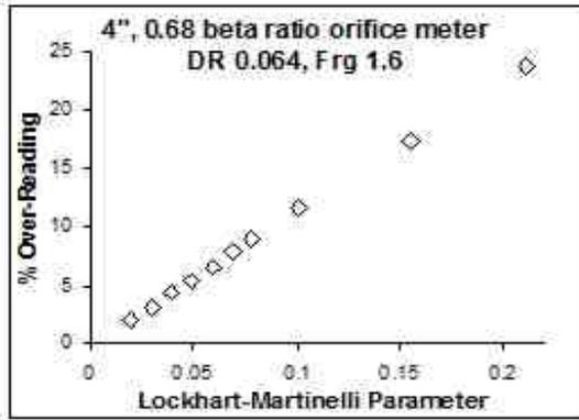
Fig 4. The Liquid Loading Effect.
