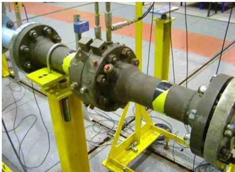
Fig 10. TUVNEL 4" Orifice Meter Wet Gas Test.
