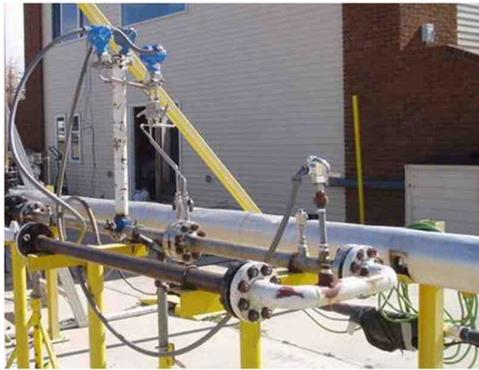
Fig 9. CEESI 2" Orifice Meter Wet Gas Test.
