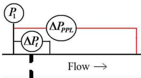
Fig 13. Sketch of Orifice Meter With Downstream Pressure Port.
