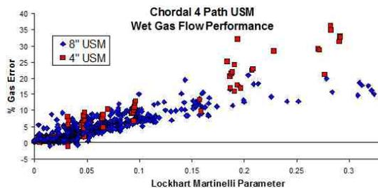
Fig 26. 4" & 8" Four Path USM Wet Gas Data.
