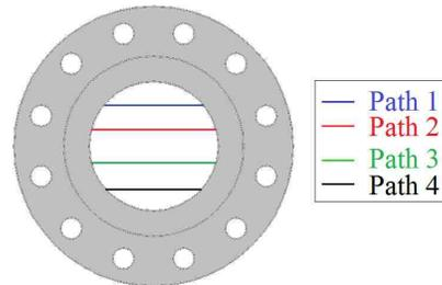
Fig 23. Sketch of a Four Chordal Path Ultrasonic Meter (not to scale)
