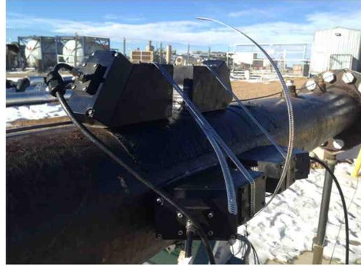
Fig 16. 8" Clamp On USM Wet Gas Tests
