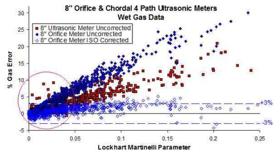
Fig 27. 8" Orifice & Ultrasonic Meter Wet Gas Data Comparisons.
