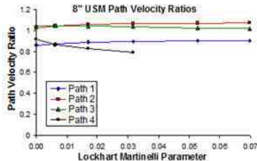
Fig 37. 8" USM Path Velocity Ratio vs.  $X_{LM}$
