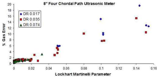
Fig 24. 8", 4 Chordal Path USM Wet Gas Data
