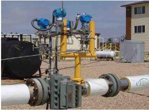
Fig 8. CEESI 4" Orifice Meter Wet Gas Test.
