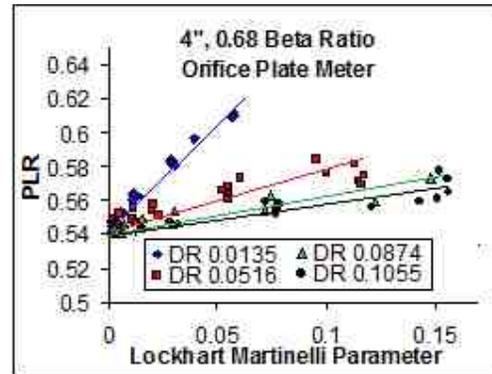
Fig 14. Orifice Meter PLR vs.  $X_{LM}$
