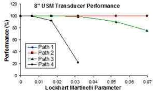
Fig 34. 8" USM Performance % vs.  $X_{LM}$
