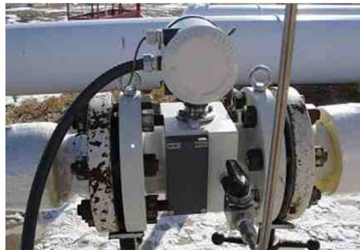
Fig 19. 4", Chordal 4 Path USM Under Wet Gas Testing
