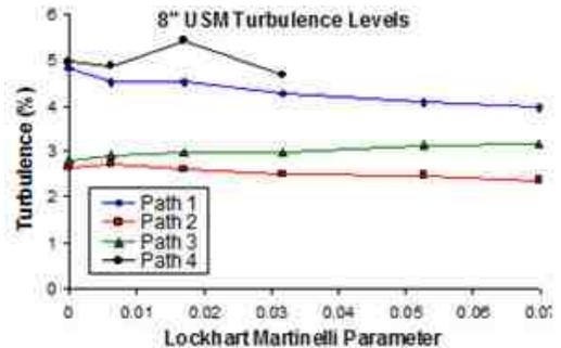
Fig 36. 8" USM Turbulence % vs.  $X_{LM}$
