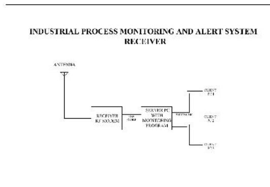
Figure 2. Receiver section for monitoring purpose at Control station
