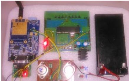
**Figure10.** *Interfacing of Arduino Development Board and RF Transceiver*
