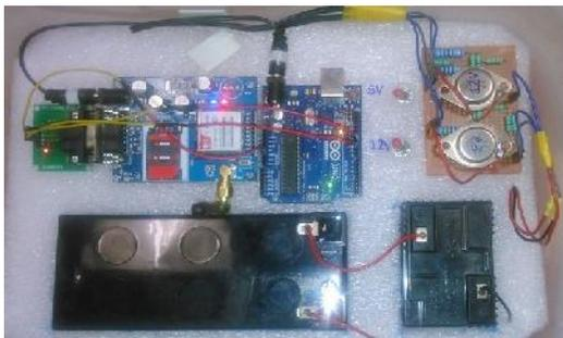
**Figure11.** *Interfacing of Arduino Development and GSM Modem*
