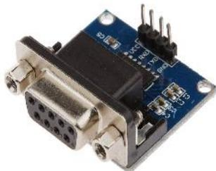
**Figure 9.** *TTL to RS232 converter*
