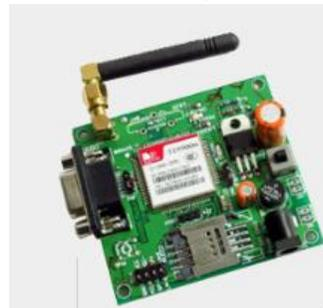
**Figure 8. GSM Modem**
