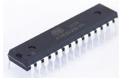
**Figure 7. ATmega328 microcontroller**
