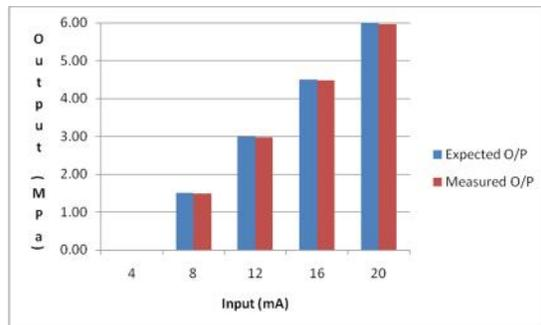
**Figure14.** Graph for Pressure Measurement
