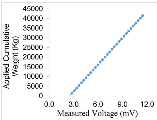
Fig. 10 calibration curve of measuring tank load cell
