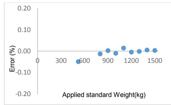
Fig. 8 Regression error of calibrator tank load cell
