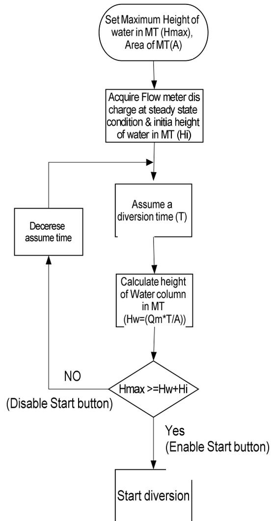
Fig. 5 Program flow chart for overflow control of water
