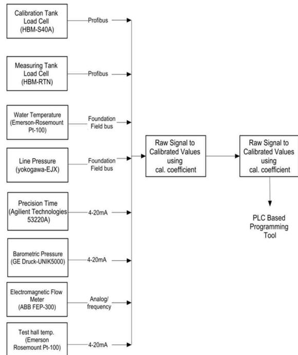
Fig.3 Data acquisition and communication to various field instruments
