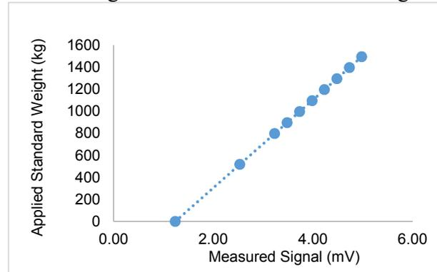
Fig.7 Calibration curve calibrator tank load cell
