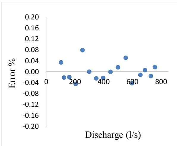
Fig.13 regression error of flow meter
