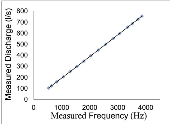
Fig.12 Flow meter calibration curve
