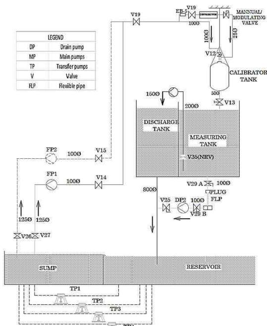
Fig.9 measuring tank load cell calibration loop
