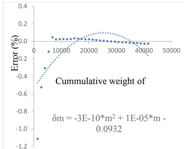
Fig. 11 Regression error of measuring tank load cell
