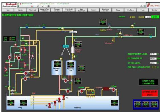
Fig.2 SCADA screen for flow meter calibration
