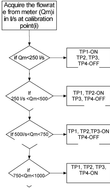
Fig. 6 Program flow chart for Sump level control
