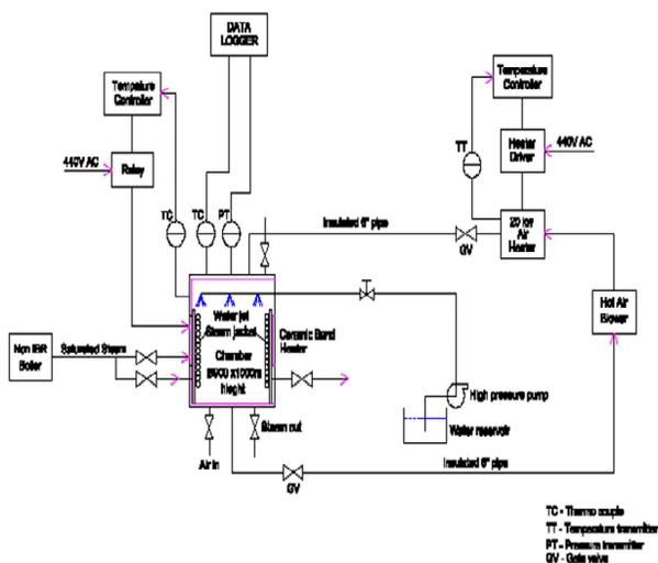
Figure.7. Schematic of MSLB test setup
