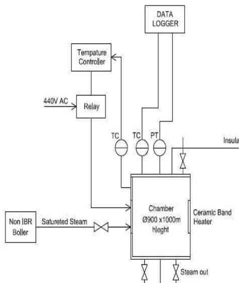
Figure.4. Schematic of LOCA test scheme
