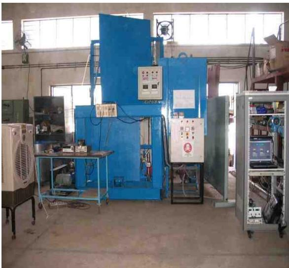
Figure.9. Photograph of HOT cycle test facility
