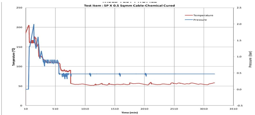
Figure 6 Temperature & Pressure Plot during MSLB test
