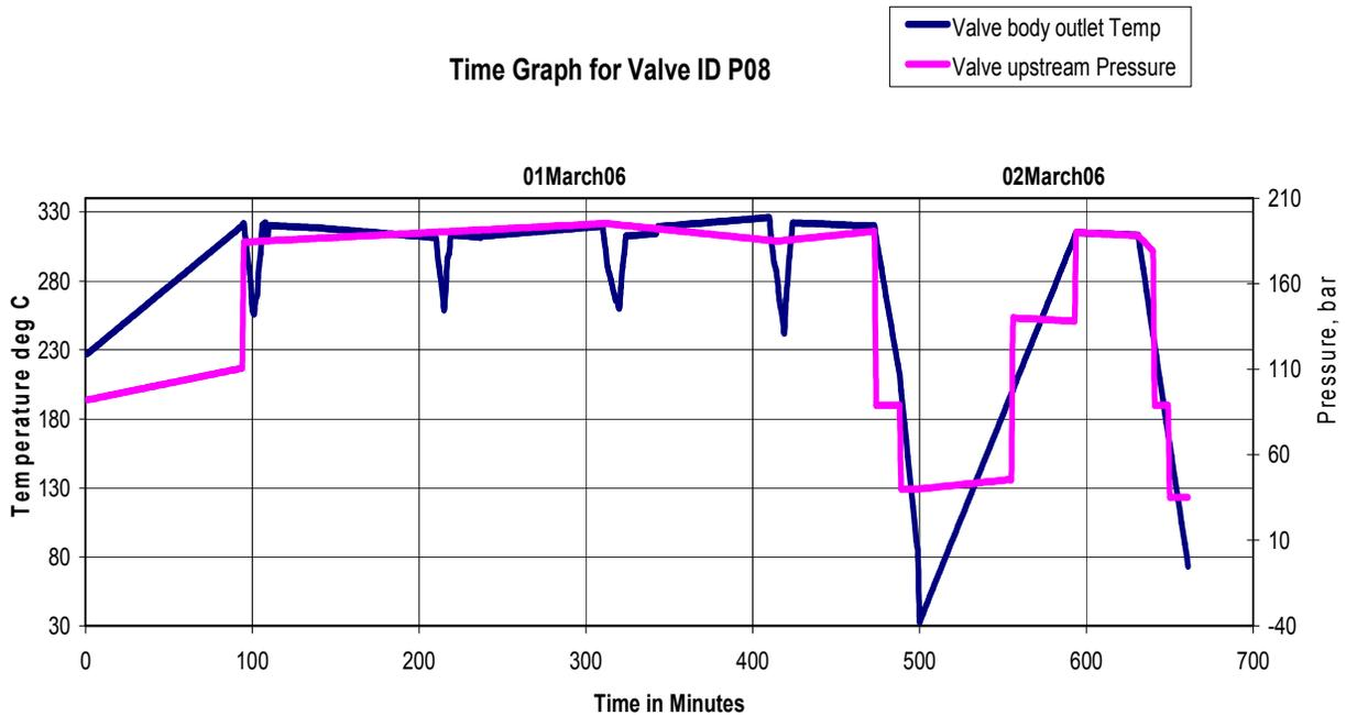
Figure 8 Time – Temperature, Pressure graph during thermal cycling test
