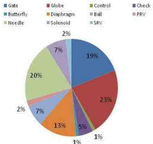
Figure.1 Population of valves for a typical Nuclear plant
