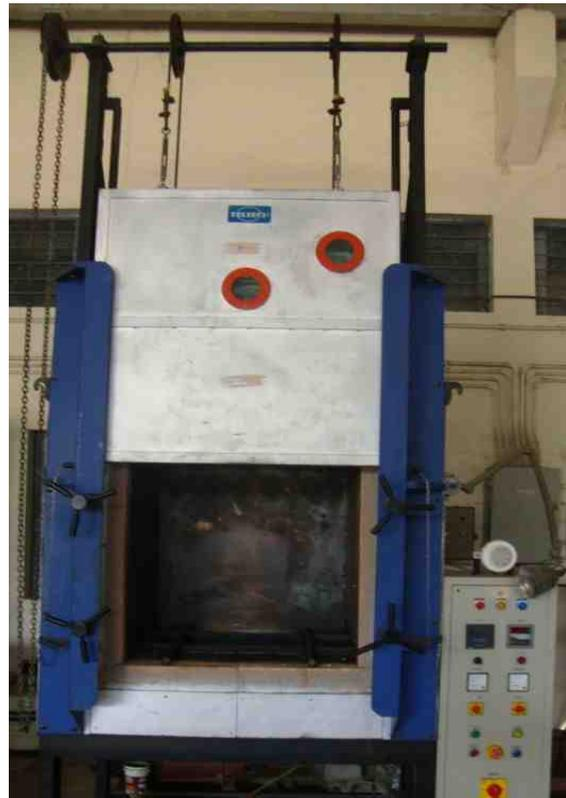
Figure.2 Thermal aging test facility
